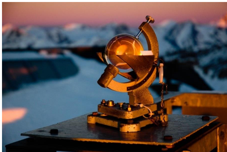
Figure 5 The Campbell-Stokes sunshine recorder at station Sonnblick.
