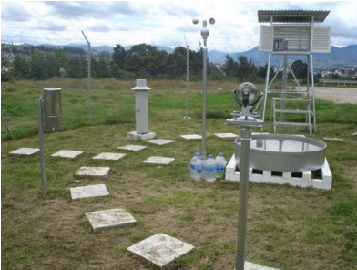
View of basic instrumentation; Official rain gauge is on the left and in silver colour
