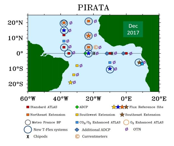
The PIRATA array in December 2019, indicating the mooring types and enhanced instrumentation that is deployed at specific sites
